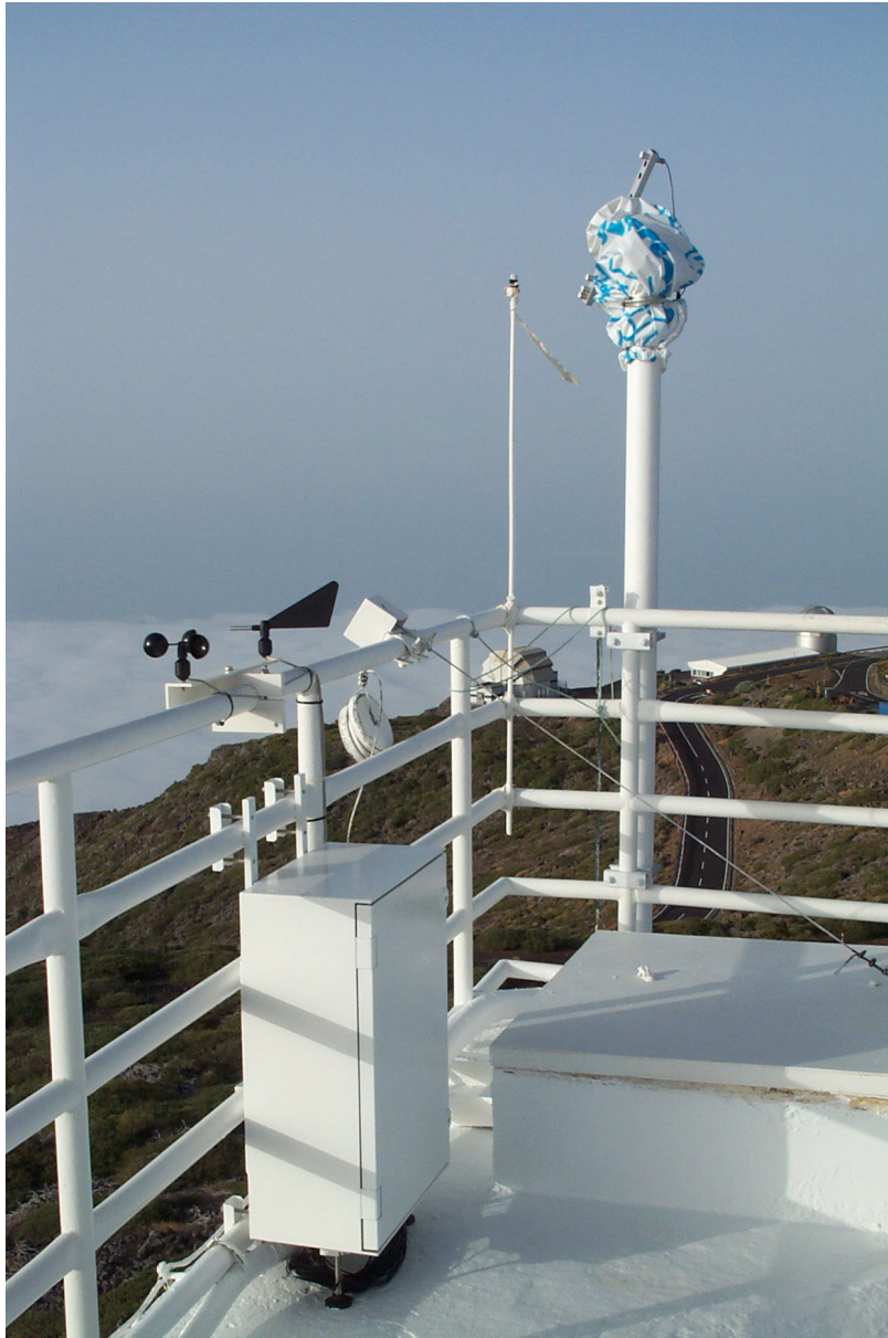
Figure 7. A SHABAR installed on the SST, on a 2 m high metal tube, with a plastic jacket covering the mount. On the fence to the left, an enclosure is mounted containing all the electronics. Only power and Ethernet cable go into the SST building.
